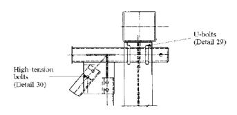
Beam-Cohmun Connection for Truss Structure Example 18
